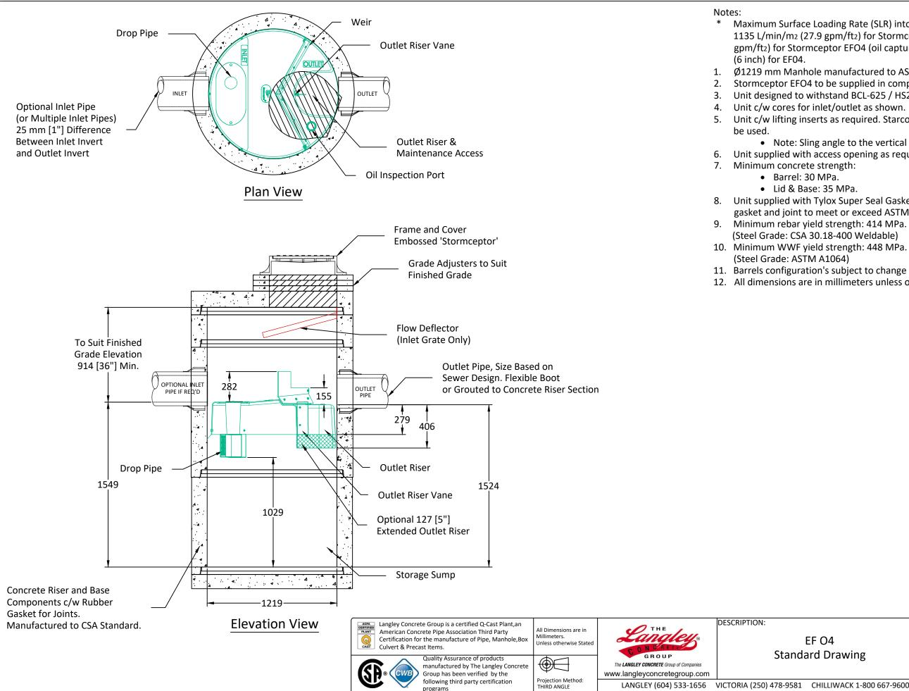
Maximum Surface Loading Rate (SLR) into lower chamber through drop pipe is 1135 L/min/m<sub>2</sub> (27.9 gpm/ft<sub>2</sub>) for Stormceptor EF4 and 535 L/min/m<sub>2</sub> (13.1 gpm/ft<sub>2</sub>) for Stormceptor EFO4 (oil capture configuration). Weir height is 150 mm
