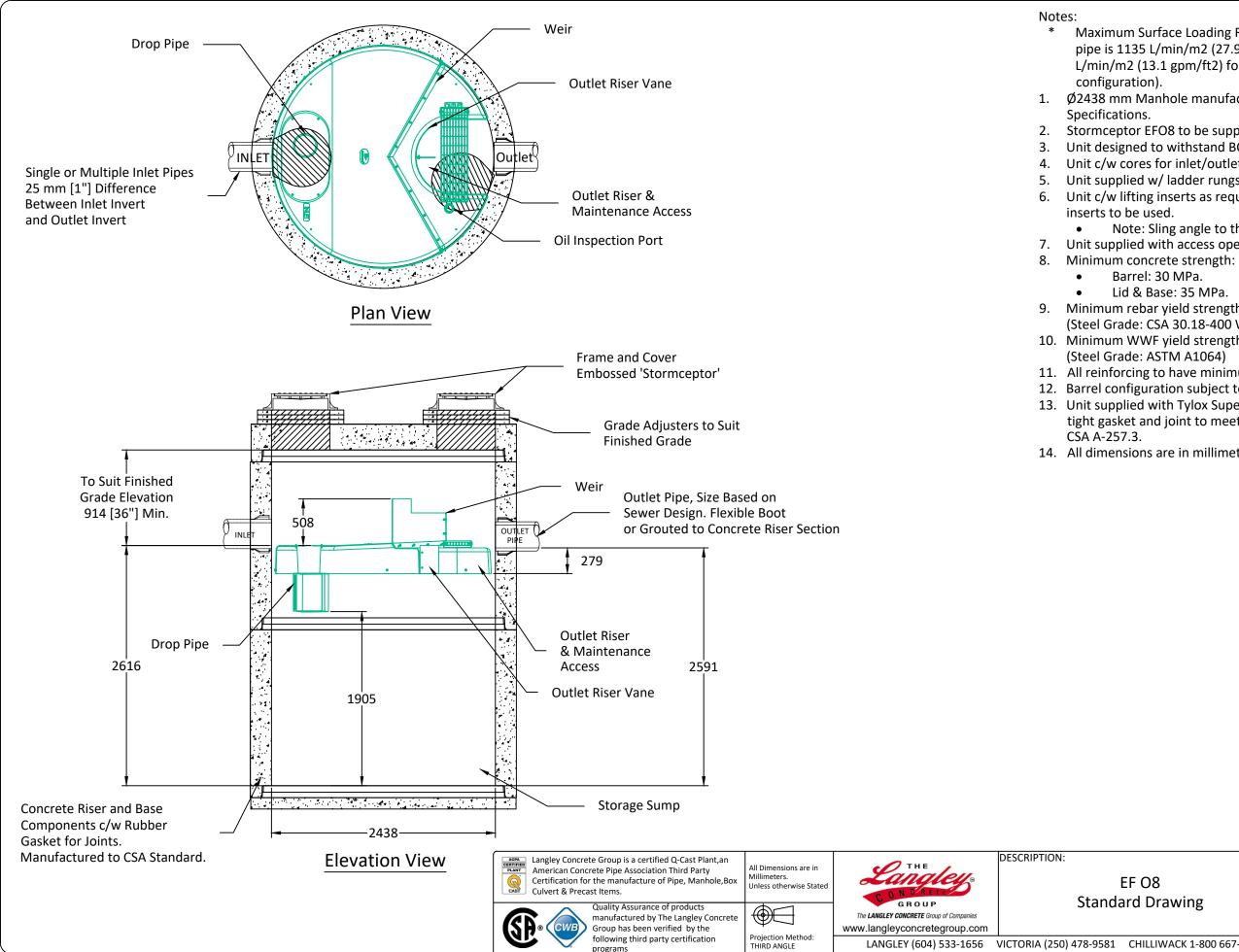
Maximum Surface Loading Rate (SLR) into lower chamber through drop pipe is 1135 L/min/m2 (27.9 gpm/ft2) for Stormceptor EF8 and 535 L/min/m2 (13.1 gpm/ft2) for Stormceptor EFO8 (oil capture
